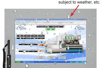
Utilizing a gasket for an environment seal provides the MCS-TOUCH with a NEMA4 rating. **Depending on** the Box Enclosure you choose, an installation can be either indoor or outdoor. A NEMA4 Box Enclosure must be used for outdoor installation or for areas that are subject to water wash-down or extreme harsh environments. The MCS-TOUCH temperature range is -20°C to 70°C / -4°F to 158°F.
